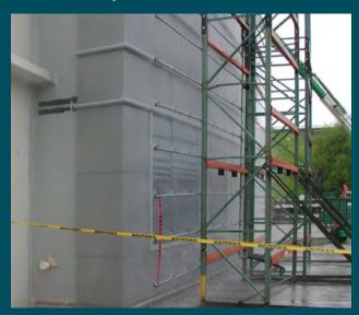
Drift or seismic joint testing in project mockup with Tremco's Proglaze ETA and ExoAir 230 Fluid-Applied, Vapor-Permeable Air Barrier Membrane.
