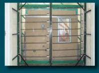
Tested to withstand **wind-driven rain** with no leaks after ASTM E331 2-hour Water Exposure test @300 Pa (6.24 psf) pressure
