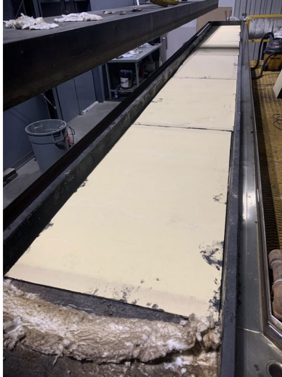
Photo No. 3 Pre-Test Unexposed Side in Tunnel
