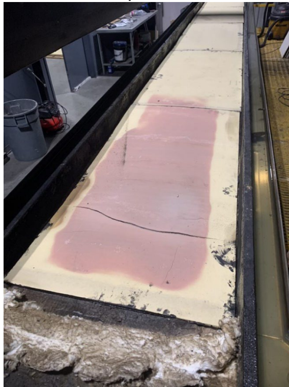
Photo No. 4 Post-Test Unexposed Side in Tunnel
