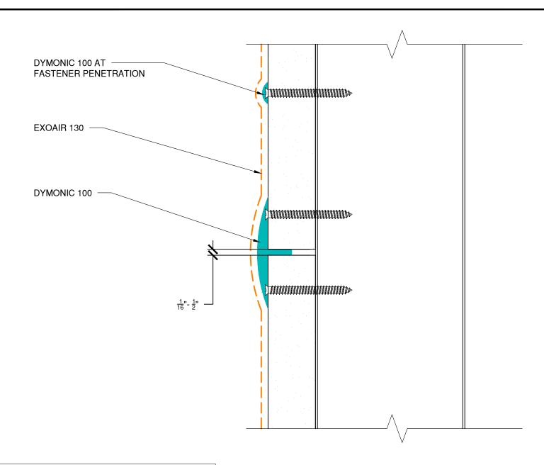
NOTE: FOR GAPS BETWEEN \$\frac{1}{8}\text{"}-\frac{1}{2}\text{"} PREFILL GAP WITH DYMONIC 100 PRIOR TO TREATING BOARD JOINT
