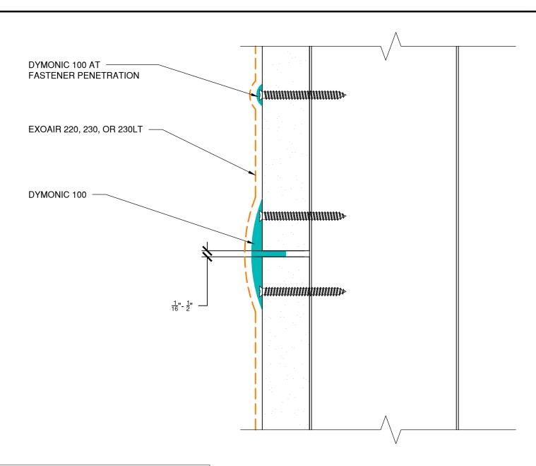
NOTE: FOR GAPS BETWEEN  $\frac{1}{8}$ " PREFILL GAP WITH DYMONIC 100 PRIOR TO TREATING BOARD JOINT
