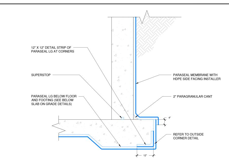
NOTE: PARASEAL PRODUCTS REQUIRE A MIN 24 PSF OF COMPACTION/CONFINEMENT IN ORDER TO FUNCTION AS DESIGNED
