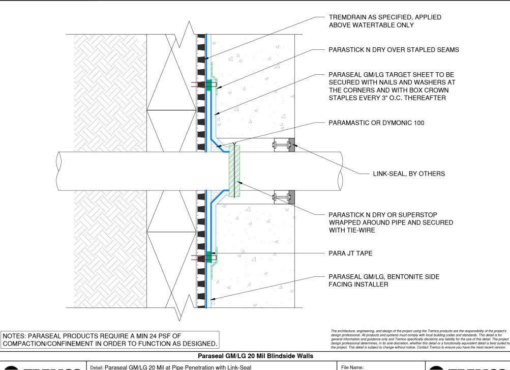
Detail: Paraseal GM/LG 20 Mil at Pipe Penetration with Link-Seal
