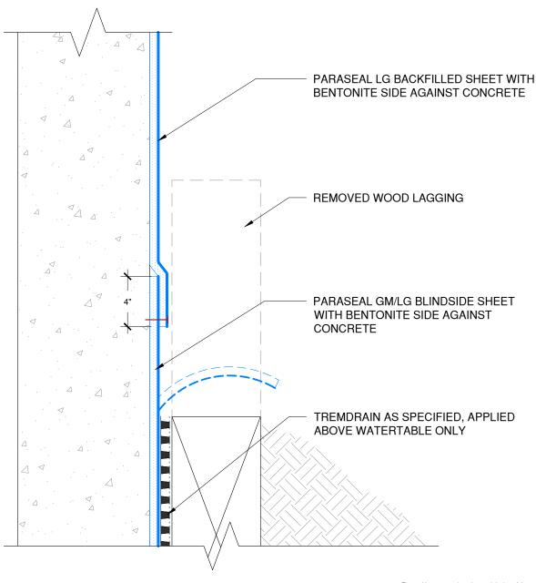
NOTES: PARASEAL PRODUCTS REQUIRE A MIN 24 PSF OF COMPACTION/CONFINEMENT IN ORDER TO FUNCTION AS DESIGNED.
