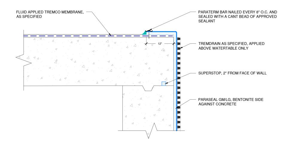
NOTES: PARASEAL PRODUCTS REQUIRE A MIN 24 PSF OF COMPACTION/CONFINEMENT IN ORDER TO FUNCTION AS DESIGNED.
