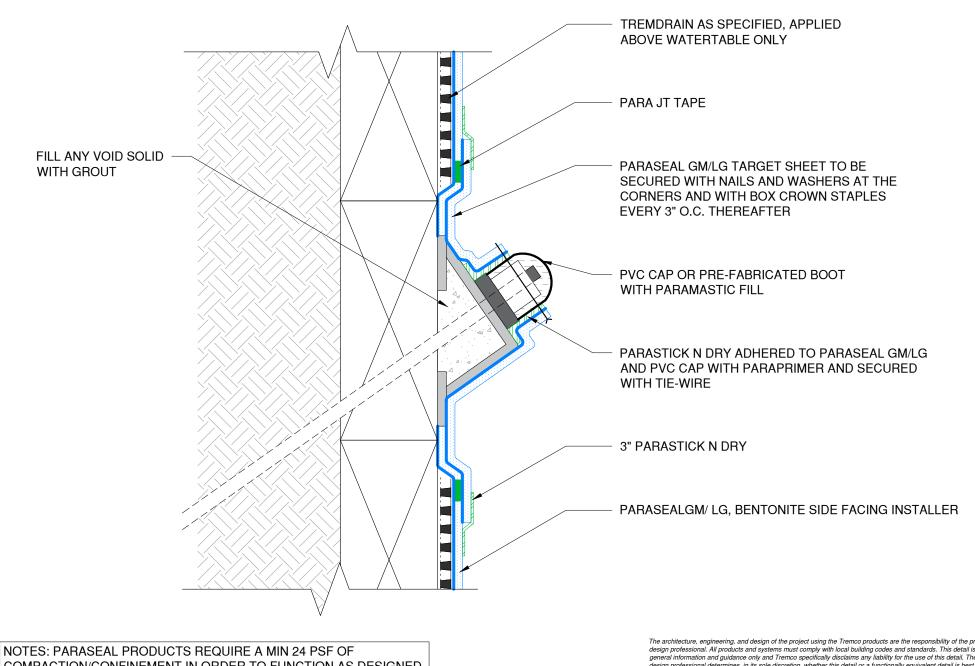
COMPACTION/CONFINEMENT IN ORDER TO FUNCTION AS DESIGNED.
