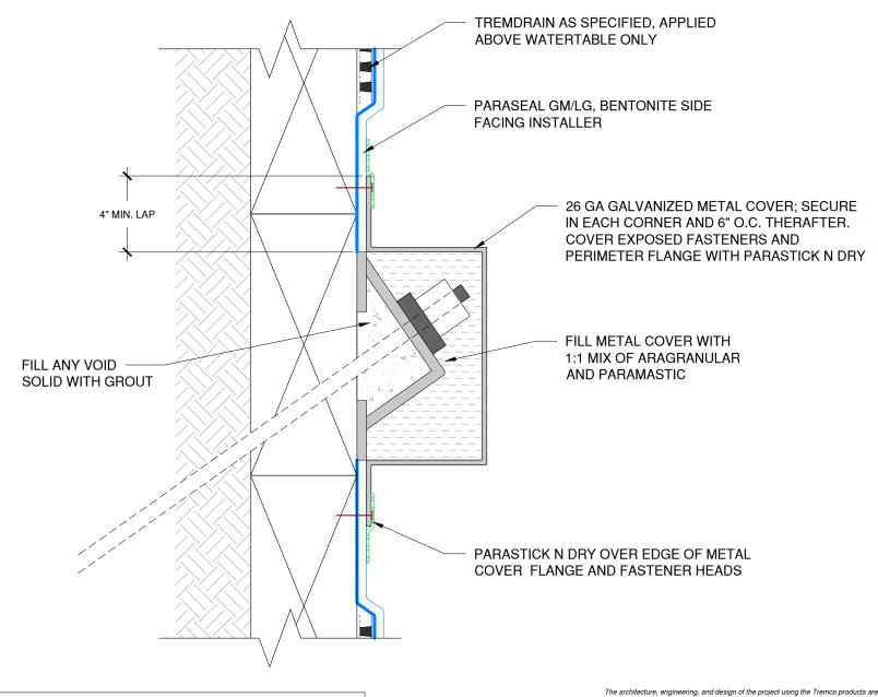
NOTES: PARASEAL PRODUCTS REQUIRE A MIN 24 PSF OF COMPACTION/CONFINEMENT IN ORDER TO FUNCTION AS DESIGNED.
