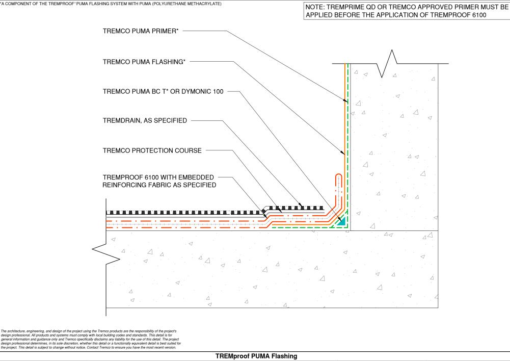
Detail: TREMproof PUMA Flashing System at Upturn - Option 2
