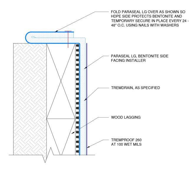
NOTES: PARASEAL PRODUCTS REQUIRE A MIN 24 PSF OF COMPACTION/CONFINEMENT IN ORDER TO FUNCTION AS DESIGNED.
